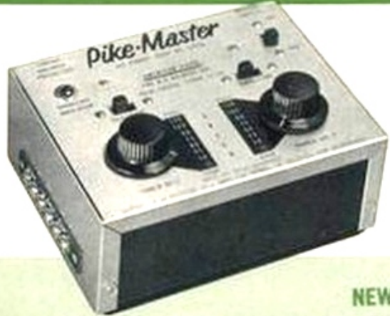
No. 32655 Twin Pike Master Power Pack. Run two trains at the same time at different speeds with this dual power pack that includes built-in thermostatic circuit breaker, two separate throttle controls and two reversing switches. Reduces 110-120 A.C. to 16 volts A.C. for accessory operation and to 12 volts D.C. for trains. $24.98
