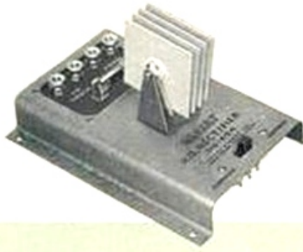
No. 32654 Rectifier. Changes A.C. from transformer to low voltage D.C. for train operation. 3 amp. output. Has reset type circuit breaker 3 3/8" high, 4 5/8" wide, 6 1/4" long. $7.98
