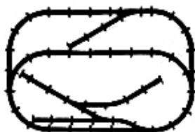
Space 68" x 90" Tracks: 23 Straight, 18 Curve, 4 - 1/2 Straight 3 pair of Switches
