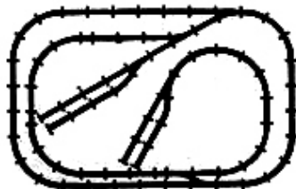
Space 70" x 110" Tracks: 28 Curve, 41 Straight, 3 - 1/2 Straight, 3 pair of Switches
