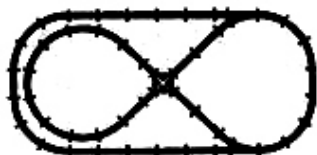
Space 52" x 108" Tracks: 21 Curve, 18 Straight, 4 - 1/2 Straight, 2 - 1/2 Curve, 1 pair Switches, 1 Crossover
