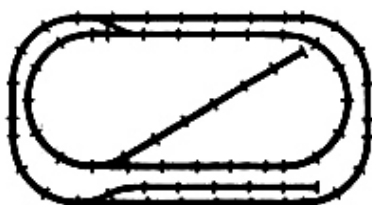
Space 60" x 108" Tracks: 31 Straight, 25 Curve, 6 - 1/2 Straight, 2 pair of Switches
