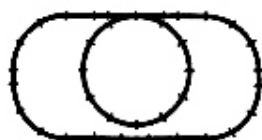
Space 48" x 96" Track: 7 Straight, 22 Curve 4 - 1/2 Straight, 1 pair of Switches
