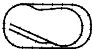
Space 48" x 96" Track: 18 Straight, 21 Curve, 2 - 1/2 Straight, 1 pair of Switches
