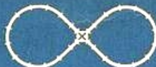
No. 6—Space 40" x 90" Track: 18 Curve, 4 Straight, 4— \frac{1}{2} Straight, 1 Crossover
