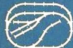
No. 26—Space 30" x 70" Track: 19 Curve, 14 Straight, 1— \frac{1}{2} Straight, 4 Left Switches, 2 Right Switches
