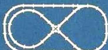
No. 5—Space 52" x 106" Track: 21 Curve, 18 Straight, 4— \frac{1}{2} Straight, 2— \frac{1}{2} Curve, 1 pair Switches, 1 Crossover
