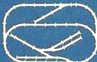
No. 22—Space 60" x 90" Track: 25 Straight, 18 Curve, 4— \frac{1}{2} Straight, 5 Left Switches, 3 Right Switches
