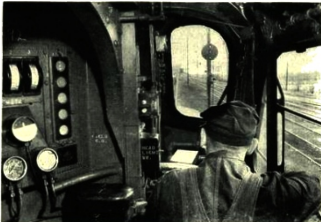
In the cab of a streamlined Electric Passenger locomotive—Note reproduction of wayside signal on panel board in cab.
