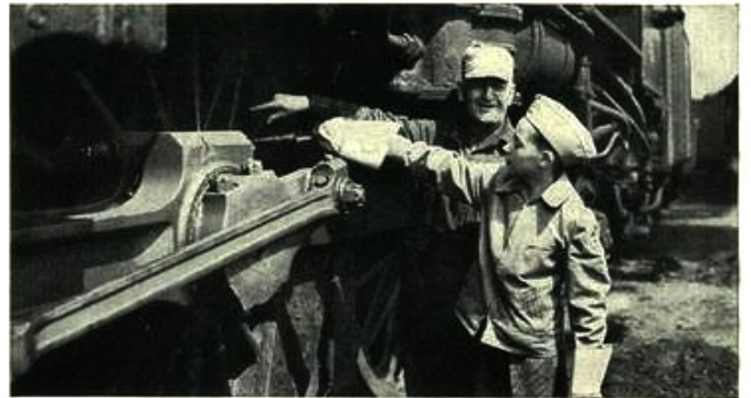
After all the inspections and servicing, the locomotive finally gets the master touch of the engineman's oil can. Here a veteran of the rails shows Jim the proper way to do the job. Now, Jim and his Dad have an appointment in the coach yard.
