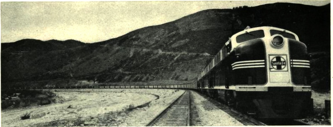
Top — Santa Fe's new 5400 H.P. freight diesel-electric locomotive, pulling the grades of Cajon Pass, California. Courtesy Santa Fe Railway
