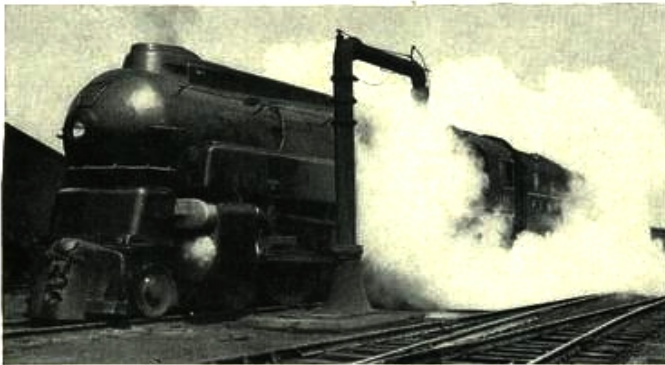
"Blowing her off" to get fresh water into the boiler of the locomotive. All the steam escaping really made a lot of noise. The locomotive is now ready for the run.
