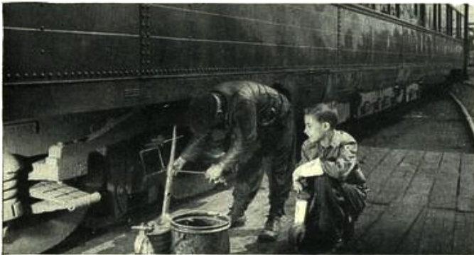
Seeing how a journal box is packed, solved a mystery. Jim couldn't understand how axles of railroad car wheels could be kept lubricated while running. Workmen put sponging in the journal box with a metal poker. Sponging is merely "waste" saturated with oil.
