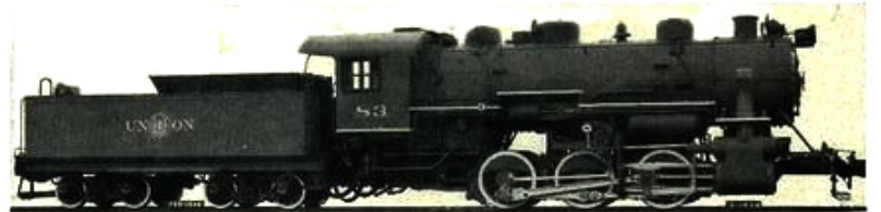
above — 6 WHEEL SWITCHER 0-6-0
