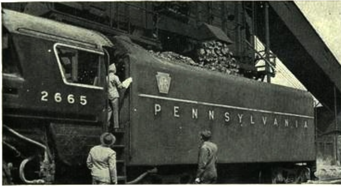
Jim stood in the cab gangway so he could see the locomotive's tender being filled with coal. Some locomotive tenders hold 60,000 pounds (or 30 tons) of coal—more than twice as much coal as Dad burns in his furnace at home in a year.
