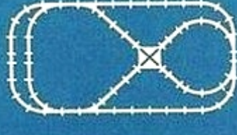
No. 20—Space 65" x 130" Track 22 Curve 4-1/2 Curve 26 Straight 5-1/2 Straight 3 pair of Switches 1 Crossover
