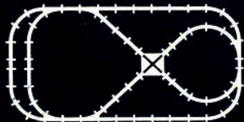
No. 20 — Space 65" x 130" Track 22 Curve 4 - 1/2 Curve 26 Straight 5 - 1/2 Straight 3 pair of Switches 1 Crossover
