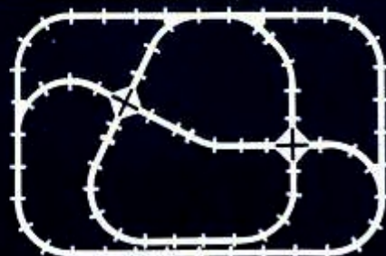
No. 16 — Space 80" x 120" Track 28 Curve 30 Straight 3-½ Straight 2 pair of Switches 2 Crossovers
