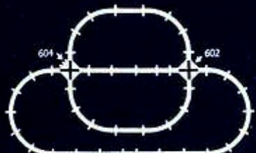
No. 1—Space 67½" x 105" Track 24 Curve 11 Straight 2-½ Straight 1 Crossover 1 Train Control Crossover THIS LAYOUT ALLOWS THE OPERATION OF TWO TRAINS AT THE SAME TIME. A TRAIN CONTROL CROSSOVER IS USED TO PREVENT COLLISIONS.
