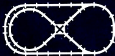
No. 5—Space 46" x 100" Track 21 Curve 14 Straight 4-½ Straight 2-½ Curve 1 Crossover and 1 pair of Switches
